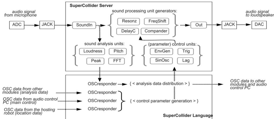
**Fig. 2.** Structure of the signal processing software SC
