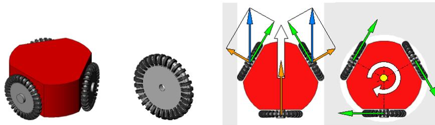
**Fig. 4.** Left: omnidirectional drive system in 120° configuration. Middle: Model of an omni wheel used in the omnidirectional drive system. Right: Omni drive with different global movements (white arrows) and the needed wheel velocities (green: propulsion velocity, orange: slide velocity, and blue: effective velocity) [15]
