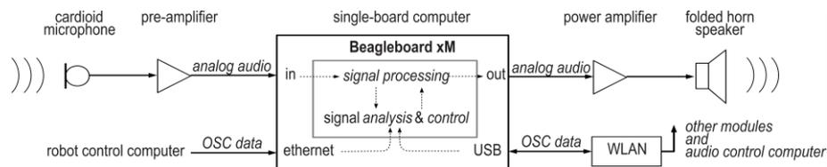
**Fig. 1.** Hardware architecture of the developed audio module.
